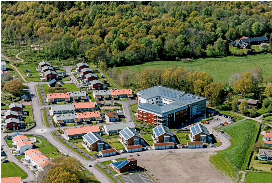
Figure 19: Aerial view on the “Vallda Heberg” residential area, Kungsbacka, Sweden (Source: Eksta Bostads AB). In sum, 570 m 2 flat plate collectors (FPC) and 108 m 2 evacuated tube collectors (ETC) roughly supply 29% of the final thermal energy demand (incl. network heat losses) of the buildings with a heated floor area of around 14.000 m 2 .
