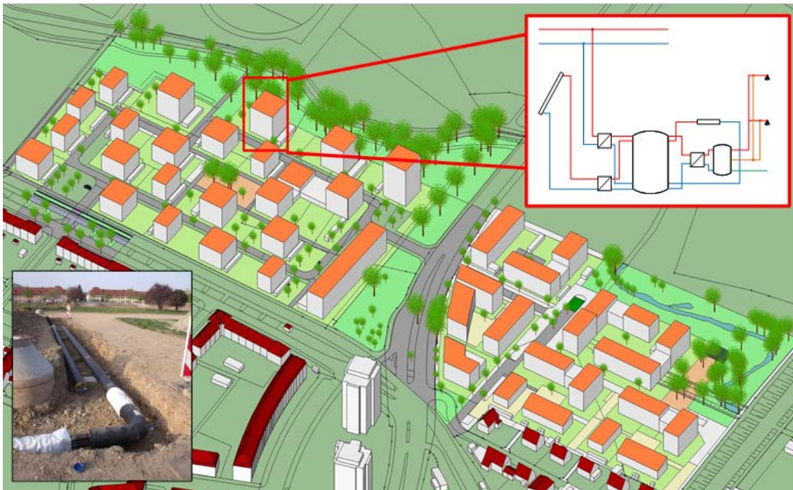
Figure 16: Development area Gutleutmatten in Freiburg i. Br. incl. principle diagram of the hydraulic solar thermal integration to the local heating grid (Source: City planning office Freiburg i. Br., Fraunhofer ISE, badenovaWÄRMEPLUS GmbH & Co. KG)
